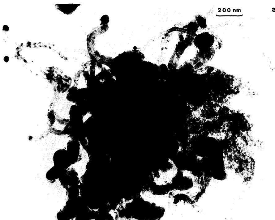
FIG. 4. Electron micrographs of the carbon deposits formed: (a) on the 10 at.% Cu catalyst (whisker carbon); (b) on the 80 at.% Cu catalyst ("octopus" carbon); (c) on the 100 at.% Cu catalyst ("pneumatic tube" carbon).
